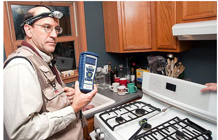
Carbon monoxide & combustion safety tests
